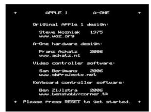
As opposed to an original Apple 1, which displays garbage after it has been switched on, the A-One will show a splash screen with some interesting URL's you can visit. You are then prompted to press the RESET switch, which will start the Apple 1, clears the screen as usual and shows the flashing cursor.
