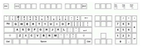
The keyboard controller expects a US layout PS/2 keyboard. Not all keys are used because they wouldn't make much sense to the Apple 1. As a bonus you can type some keys which could not be typed on an original Apple 1 keyboard (e.g. the square and curly brackets). In order to avoid confusion the keyboard controller can only generate upper case characters.
